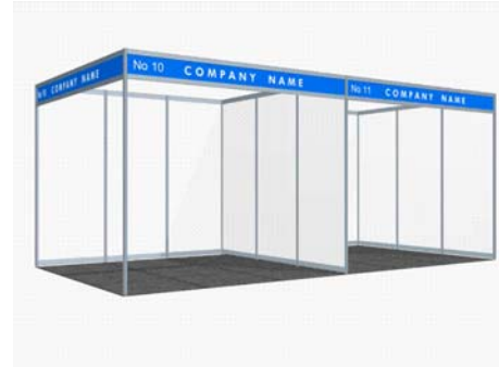
Diagram of standard 3m x 3m shell scheme
